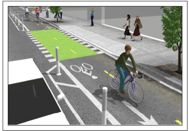
Illustration of a two-way Protected Bike Lane
